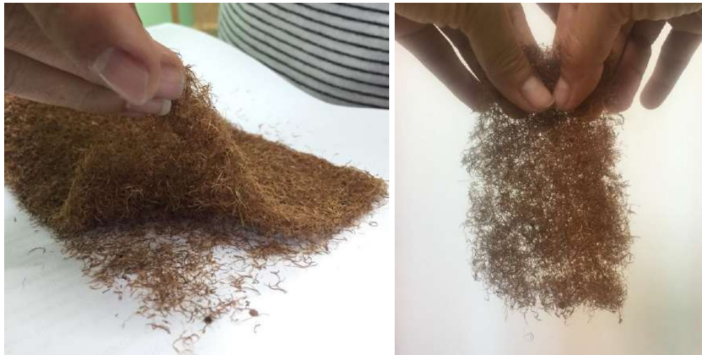
Figure 14: Blanket disintegrated after handling
