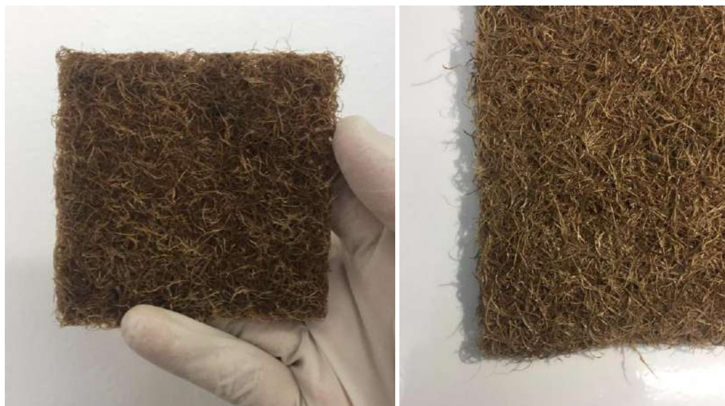
Figure 16: Non-woven fabric with consolidated açai fibers
