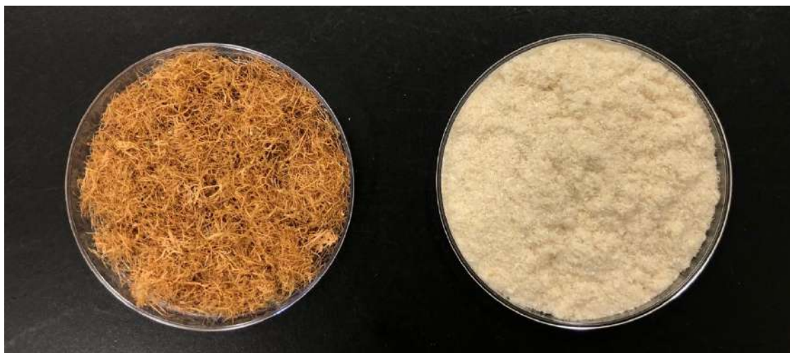
Figure 05: Samples of raw açai fiber and samples of bleached fiber
