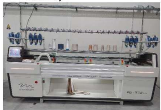
B Electronic Knitting machines - Mandarin, Full Garment Series (FG372 STF - Smart Yarn Feeders)
