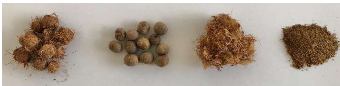
Figure 04: Mixed waste; pits; fibers and açai grounds - respectively
